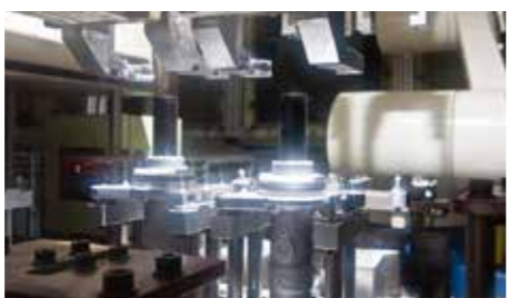
Master cylinder assembling 制动主缸组装线
